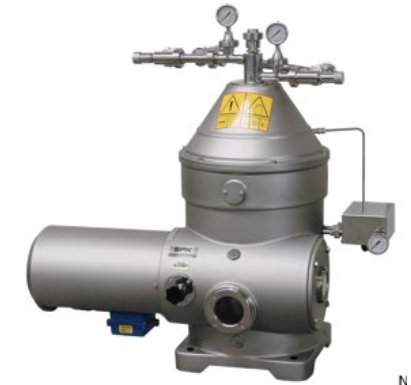
SE06V-X Solid bowl warm milk separator Warm milk skimming capacity: 2000 l/hr Milk standardisation capacity: 300 l/hr 5.5kW 4-pole motor, Bowl speed 7500 rpm
