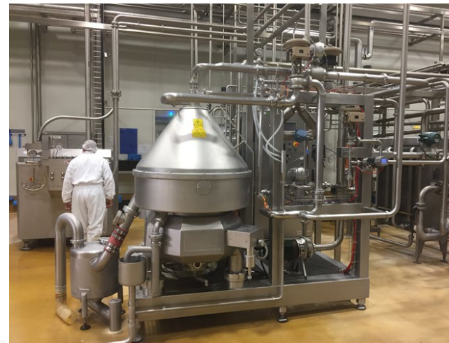
SE60X-Q3P3 Self-cleaning warm milk separators Skimming capacity : 20,000 lit/hr
